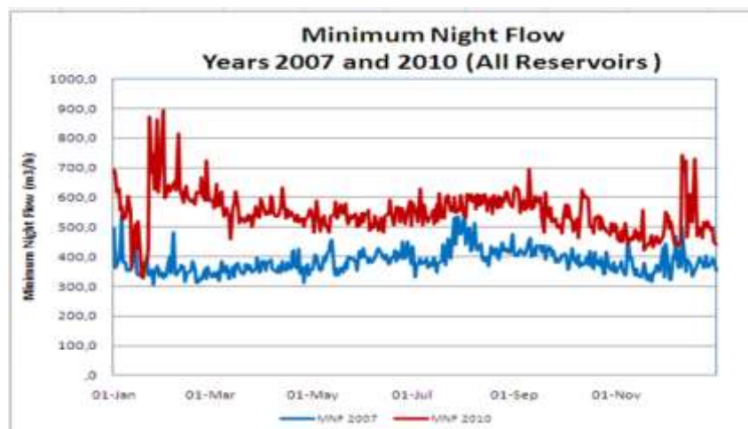
Figure 4 Minimum Night Flow before and after IWS
